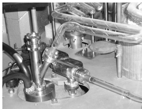
Fig. 4 A general view of the inner vacuum system for the extraction of noble gases
