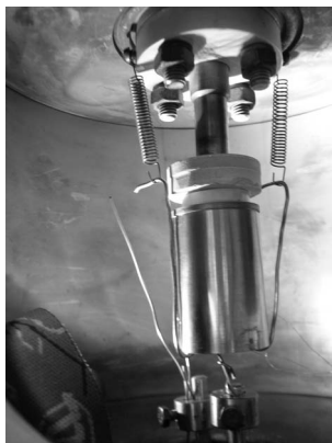
Fig. 1 The tantalum–titanium crucible with newly designed heating unit installed in the external vacuum chamber, a view through CF 100 access flange
